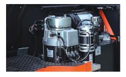
Low-noise gear pump ensures quite lifting. Motor controller, oil pump motor controller and steering motor controller, provide self-protection, maintenance-free, superior performance.
