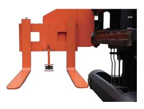
A strong chassis and optimized center of mass distribution ensure excellent stability. High-precision transverse slide rail with excellent gap compensation enhances transverse slide stability. When the forklift reaches the maximum height, the height limit function automatically cuts off lifting power to provide safe lifting. Speed limit controls automatically adjust during turns, adding additional safety while turning.
