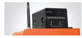
The dual-screen, 3-camera, high-definition monitoring system allows the operator to monitor cargo stacking in real time.
