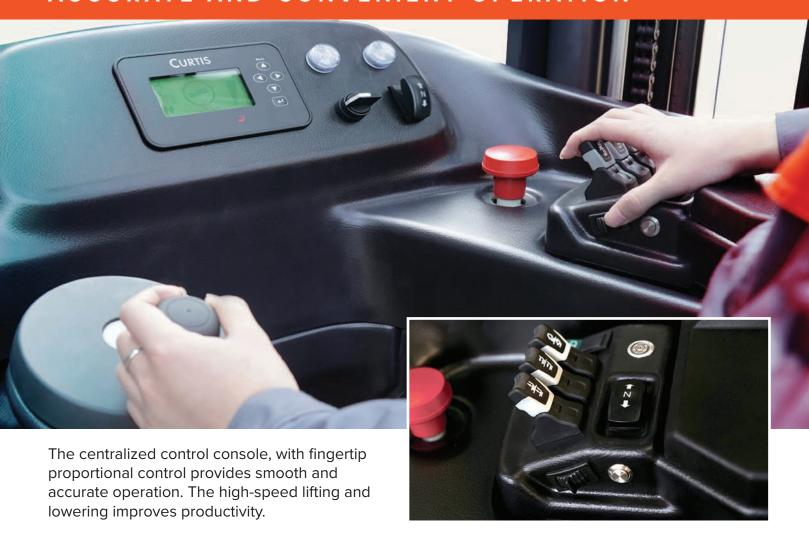
The steering wheel and central control console can be adjusted freely in all directions for maximum operator comfort.
