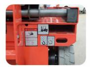
Standard transportation forklift holes and crane holes
