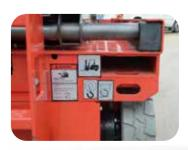
Standard transportation forklift holes and crane holes
