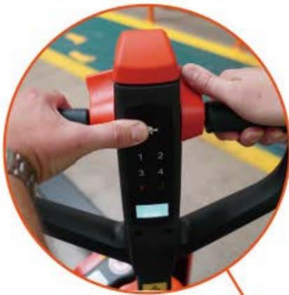
The ability to operate the unit with the tiller in the upright position allows working in confined spaces.
