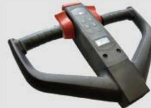
Tiller is made of fiber glass material for high strength.
