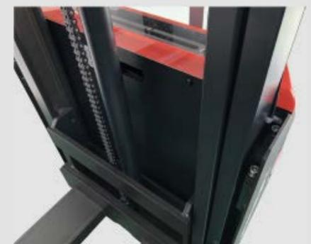
Support legs are made out of solid steel (not tube) to have enough rigidity to ensure the stability and safety.
