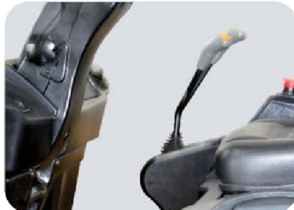
Ergonomic Right Hand Operating Hydraulic Handle
