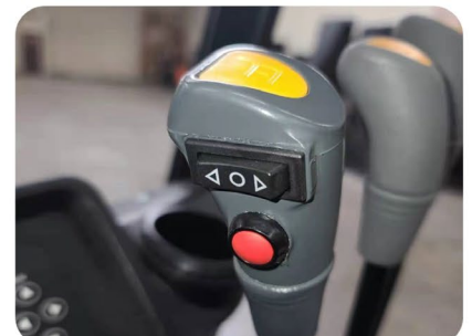
Forward / Reverse Switch on Handle
