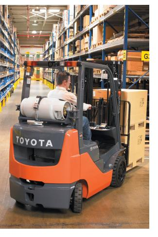
IC forklifts only require storage space for propane tanks. They're also suitable for both indoor and outdoor applications. This is particularly useful for situations that involve moving materials in and out of a facility. Advancements are being made to make electric forklifts more suitable for outdoor use. For example, Toyota's three-wheel electric and 80-volt pneumatic models were designed to protect critical forklift components from potential damage due to water intrusion.
