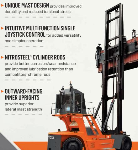
STANDARD SIDE-POST ATTACHMENT extends/retracts to handle 20- and 40-foot empty containers, and can be quickly adjusted to handle 53-foot containers
